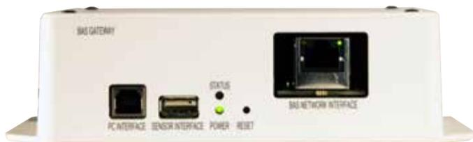
**Wireless Gateway - Interface Ports and Status LEDs**
